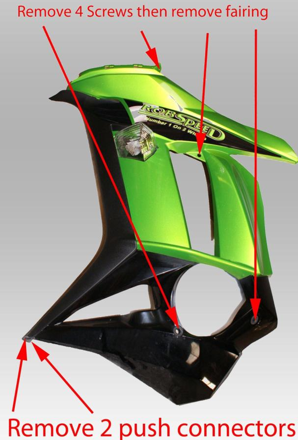
2. The fairing has retaining clips at the top of the fairing. The fairing will need to be pulled backwards then outwards to allow removal. Disconnect indicator before full removing fairing. Please see Diagram
